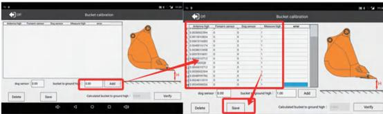
Note: When the stick is in different positions, ensure that the bucket does not touch the ground during rotation.
