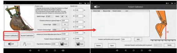
② Technicians need to measure the vertical distance from the ground to the connection point between the stick and the bucket, as depicted in the figure.
