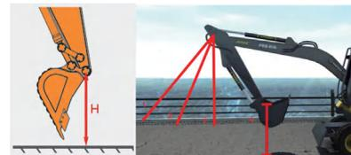
③ Technicians should enter the measured height into the calibration interface each time, and then proceed to measure the next height. This process should be repeated at least four times before clicking the Save button to complete the stick calibration.
