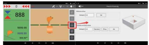
Step 1: Position the bucket appropriately and click the Reference Surface Setup button.
