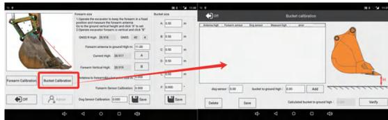
② Technicians are required to measure four sets of data, with each set consisting of four measurement results, totaling 16 results.
