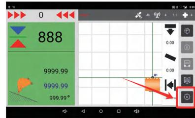
Click the User button, then enter the password: 1, in the password box, click Confirm to unlock the calibration content in the interface.
