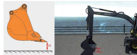
Technicians should enter the measured height into the calibration interface each time, and then proceed to measure the next height. After measuring all 16 parameters, click the Save button to complete the bucket calibration.
