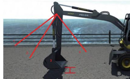
Each set of data requires measuring the distance from the bucket to the ground four times at different bucket angles.
