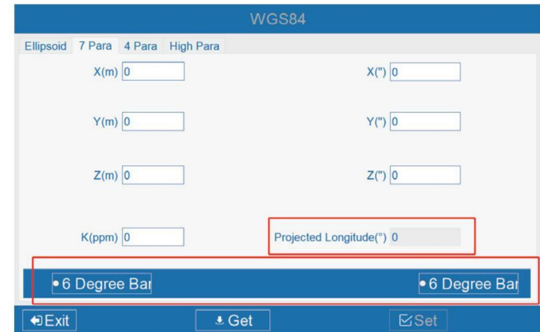
Figure 6 7-Parameter and Central Meridian & Zone Settings
